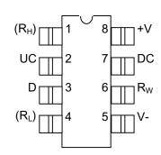
8-Pin SOIC (208-mil) See Mech. Drawings Section
